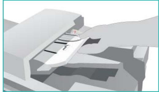
2. Lift up the *document feeder*. Place the document face down onto the *document glass* and register it to the arrow at the top right rear corner. Close the *document feeder*.
